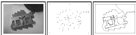
Figure 2. 2-D localization results (right) using point features (middle)
