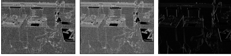
Figure1. Comparison of the results of the tracing operator for a gray value image (left) and a color image (middle); the interest operator for tracking color point features in horizontal direction (right)
