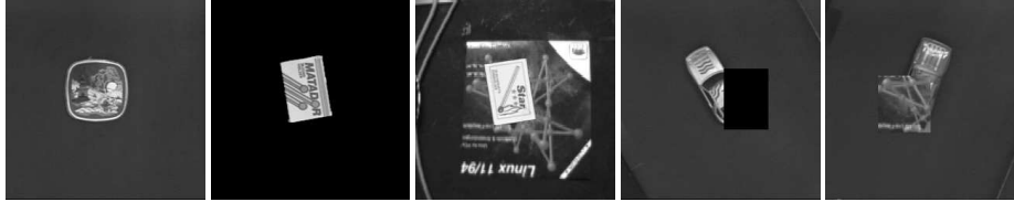
Figure 3. The 5 objects in the different environments: box on the training background, matchbox 1 on the black background, matchbox 2 on the heterogenous background, car 1 with 25% black occlusion, car 2 with 50% heterogeneous occlusion
