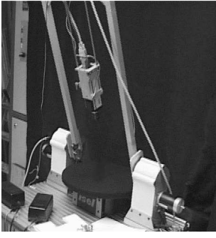
Figure 1: Experimental setup consists of turntable/arm combination. The possible pose space is defined by the azimuthal ^1\varphi^n and the latitude ^2\varphi^n .
