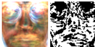
Fig. 3. The left image is an average of faces projected to different eigenspaces. This image binarised with a threshold \theta = 135 can be seen on the right side. All white pixels are deleted before classification.
