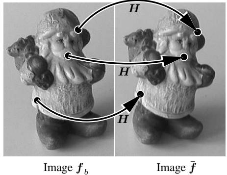
Figure 2: Illustration of the translation of the tracked feature points (marked as circles) using the homography matrix  $H$
