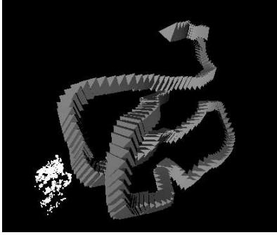
Figure 1: Camera pose and 3-D point reconstruction of the *santa* sequence with 207 images. Cameras are depicted as pyramids with their bases facing in viewing direction.
