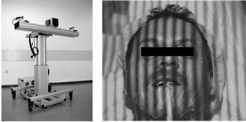
Figure 1. Left: Optical 3D-Sensor (phasemeasuring triangulation) built up by a light-source with a projector (active illumination) and two cameras bedded on an adjustable and moveable tripod. Right: A sinusoidal stripe pattern is projected onto the patient's face and measured by the cameras.
