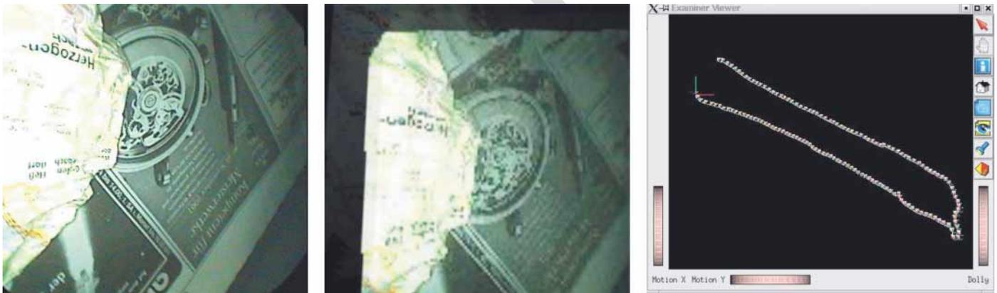
**Fig. 5** Sequence ALF029: original endoscopic image (left image), rendered image from the generated light field (middle image), calculated extrinsic camera parameters (right image, the pyramids represent the camera poses)
