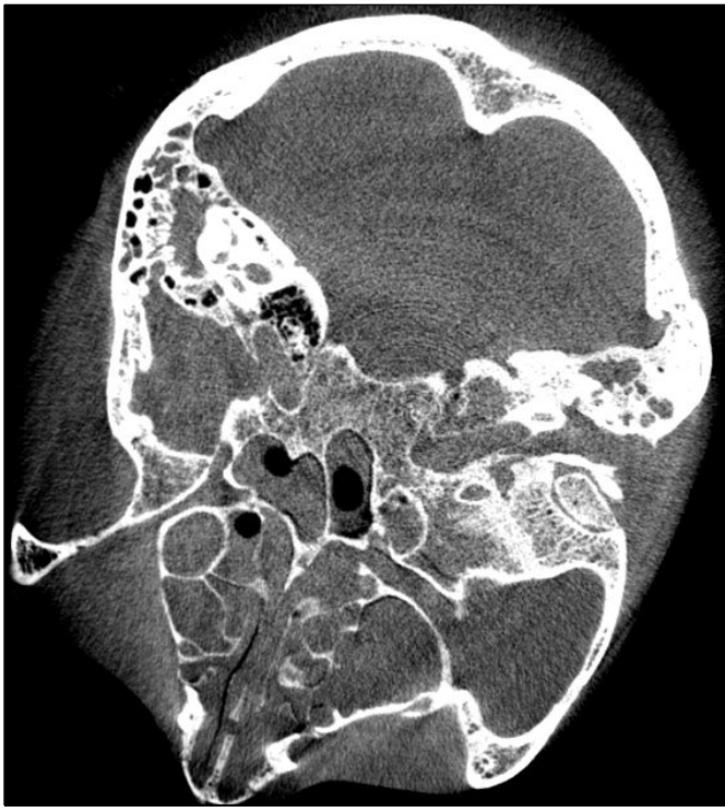
Fig. 8. Reconstruction of a human head phantom from real CB data. The slice is 53 mm away from the plane of the circular scan. The window was set to C=0 HU, W=1000 HU.
