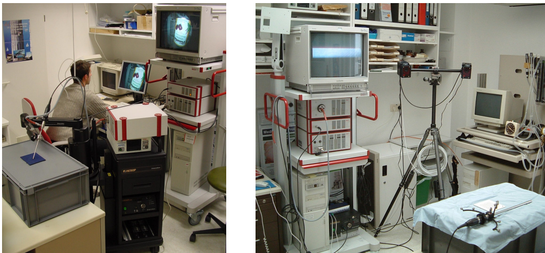
Figure 7.1: Experimental setup in the laboratory using the robot arm AESOP (left) and the optical tracking system smARTtrack1 (right). Additionally, the video-endoscopic system is visible in both images as well as the box that is utilized as an artificial patient (cf. Figure 7.2).
