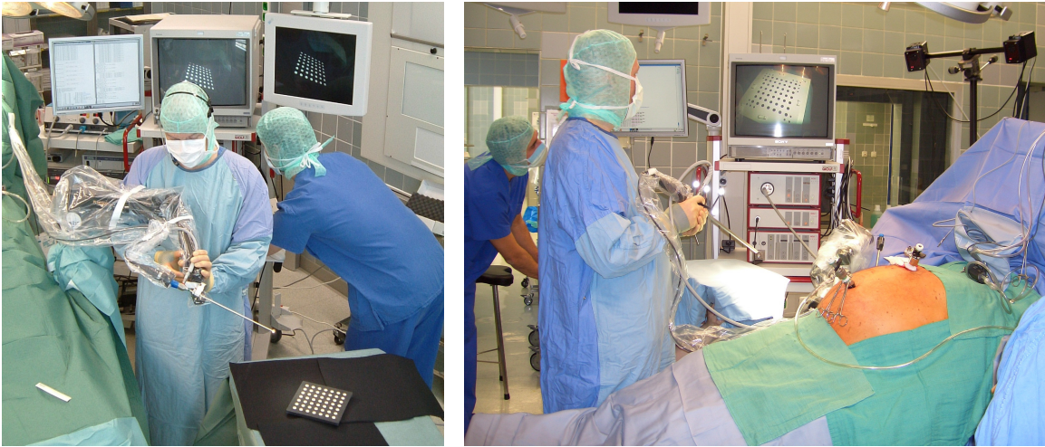
Figure 7.5: Hand-eye calibration of AESOP (left) and smARTtrack1 (right). The calibration pattern is placed on an unsterile table next to the sterile patient. The surgeon moves the endoscope for the acquisition of calibration images.
