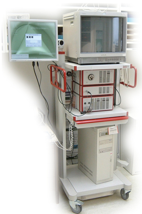
Figure 4.1: The real-time endoscopic image enhancement system: a typical video-endoscopy system on a rack is extended by a PC and a second monitor (on the left-hand side of the originally contained monitor, fixed with a positioning arm) to display the original and the processed image at the same time.
