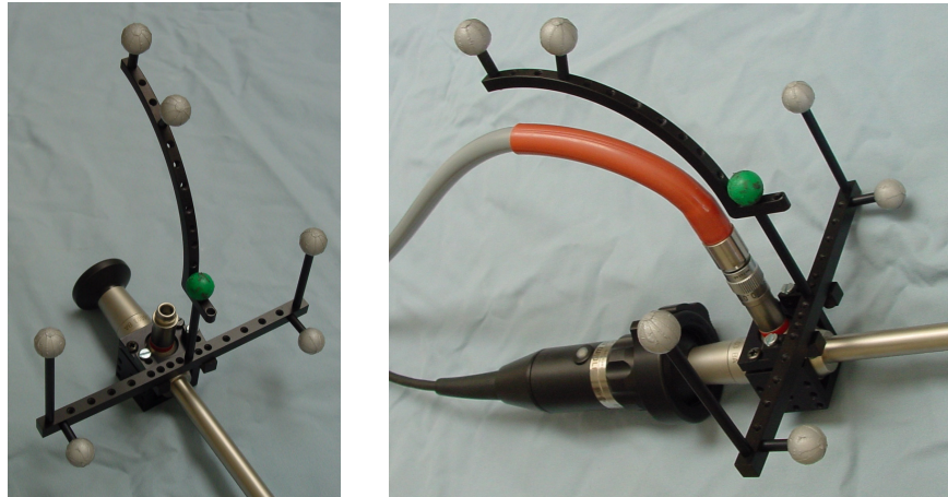
Figure 5.12: The double decker 2z target. Four markers lie approximately in the same plane. Additionally, the middle arc of the epee target was moved in front of the light conductor and two markers are placed at the end of it to provide higher pose accuracy in the direction towards the endoscope tip. The marker at the bottom of the arc is used for fixating the arc, the retro-reflective surface was removed which makes the marker invisible for smARTtrack1. The left image shows the target without camera head and light conductor whereas on the right side both are mounted.
