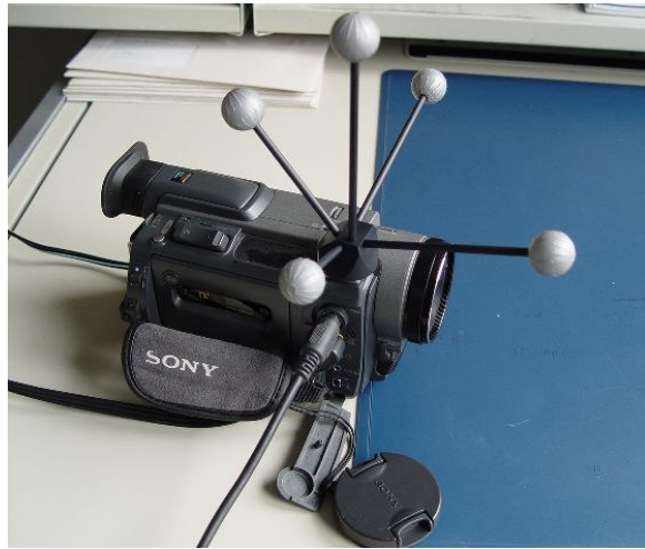
Figure 7.16: A target was attached to a conventional video camera (Sony 3-CCD) in order to test the transferability of the developed methods for light field reconstruction. The result of the reconstructed light field is shown in Figure 7.32, page 187.
