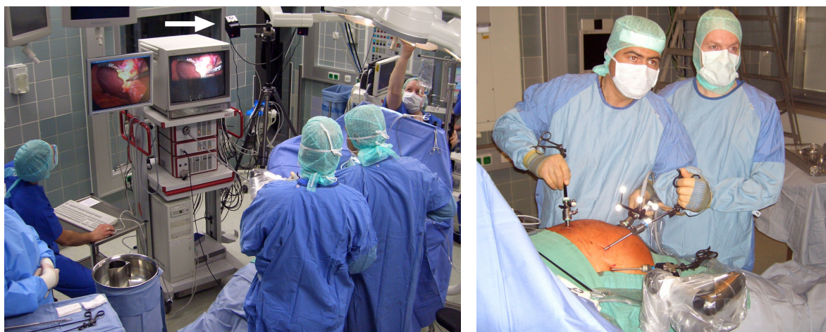
Figure 7.4: Setup in the operating room for light field reconstruction using smARTtrack1 during a minimally invasive operation (cholecystectomy). The left image shows the arrangement of the extended video-endoscopic system and smARTtrack1 on its tripod (marked by an arrow). Only the left of the two cameras of smARTtrack1 is visible. Two surgeons stand at the operating table and the author of this thesis is sitting at the keyboard. The image on the right shows the two surgeons in action, where the endoscope with the attached target is moved by the surgeon on the right side, below the arm of the surgeon on the left side.
