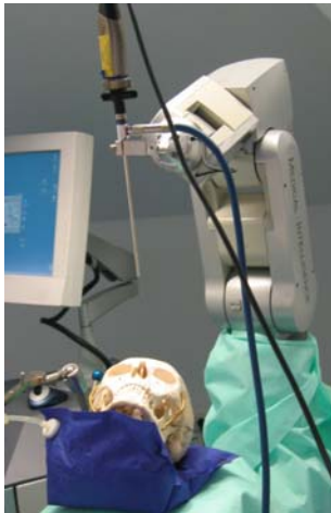
Image 2: Overview of laboratory scanning setup including the skull, the robot and the rigid endoscope
