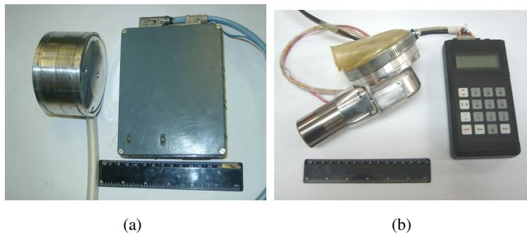
Fig. 3: Exterior of LVAD mechatronic unit: a – unit with rollerscrew mechanism; b – unit with planetary screw gear and rack
