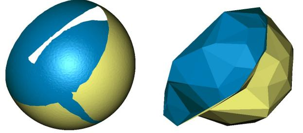
Figure 2. Reconstructions of negative half sphere, results from NBV planning approaches with ([13], left) / without ([6], right) active illumination. Whole object observed by 8 / 10 views.
