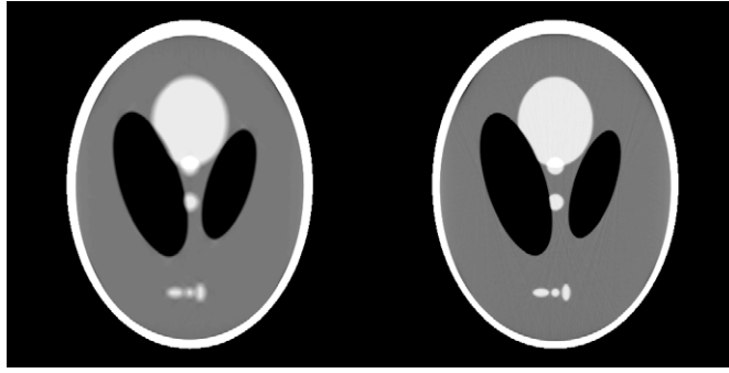
Figure 7. Reconstruction of the Shepp–Logan phantom from fan-beam data on the square-shaped source trajectory. (Left) The split chain-rule scheme. (Right) The new scheme with \varepsilon = 0.125 . The grayscale is compressed on the interval [1.012, 1.032] .
