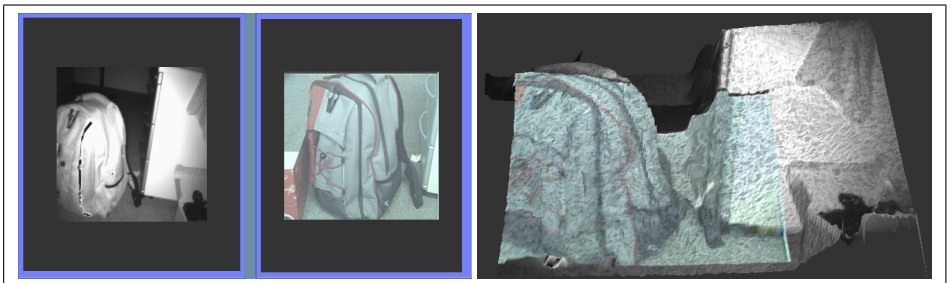
Fig. 2: Simultaneously acquired TOF and Web camera data (left image). Overlay of color information and 3-D surface reconstruction after registrating TOF and Web camera (right image). Only parts of the reconstruction can be overlaid with color information as the common field of view of both cameras is not 100% overlapping.
