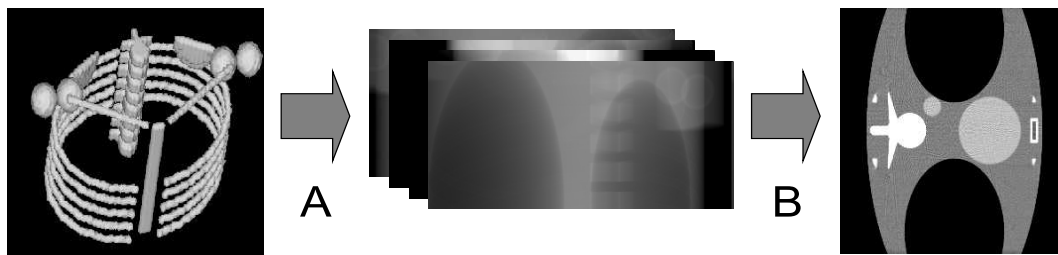
Figure 1.1: The principle of computed tomography. (A) An X-ray system acquires projection data from the investigated object that is shown on the left (3D illustration from [3]). (B) The sequence of projection images is then converted into a structural representation of the initial object using a CT reconstruction algorithm.
