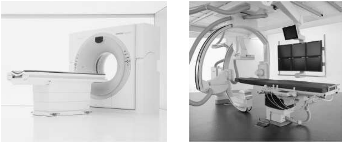
Figure 1.2: Examples of X-ray CT systems commonly used in the clinical environment. (Left) A diagnostic CT scanner from the Siemens SOMATOM Sensation family [5]. (Right) A medical C-arm device from the Siemens AXIOM Artis family [2].
