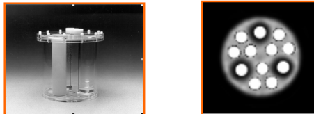
Figure 2. Data Spectrum NEMA 3 cylinder phantom and the region of interests (ROIs) generated by MiQ phantom analysis tool.
