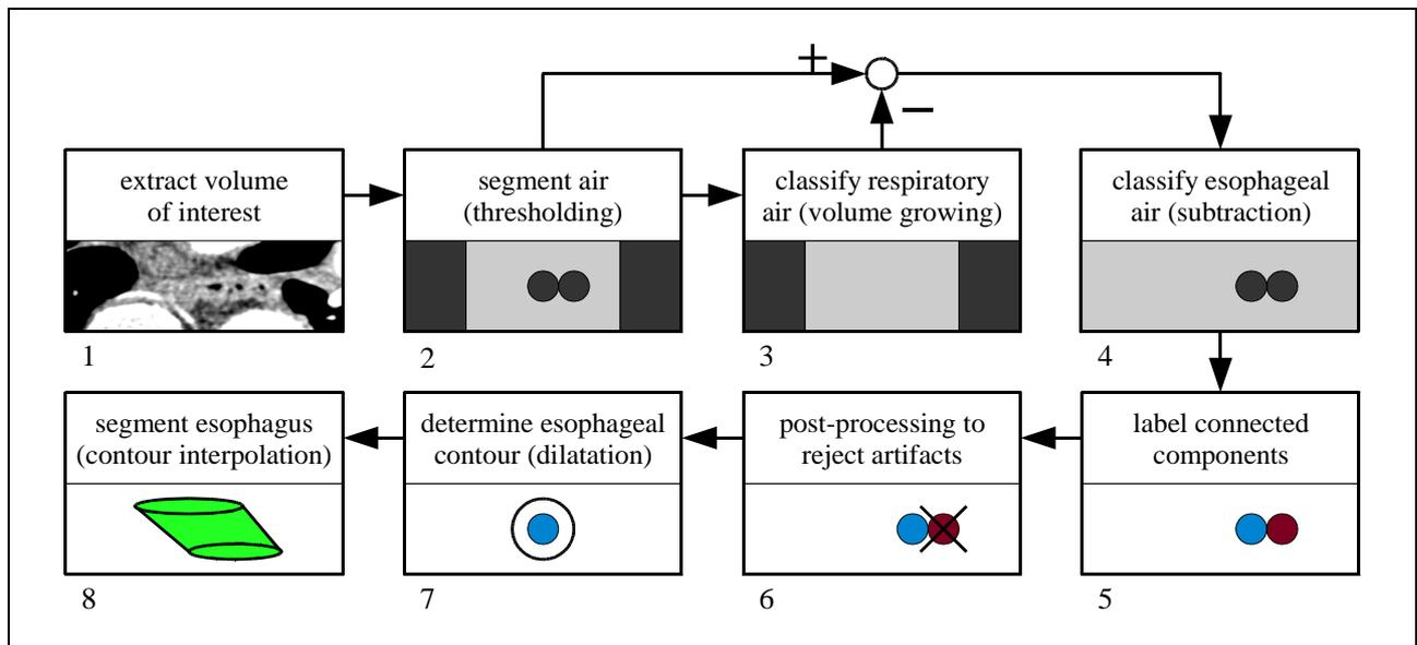
**Fig. 1:** Flow chart of the algorithm for automated 3D esophagus segmentation in CT images
