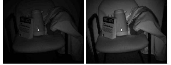
Figure 6. Image with specular reflections. On the left the original image, on the right the intensity-corrected one.
