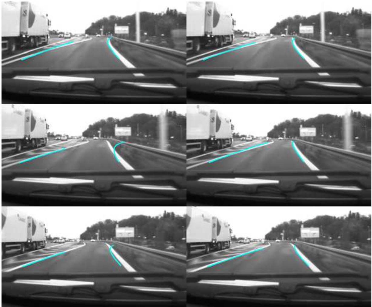
Fig. 3: Feature selection without (left) and with map constraints (right).
