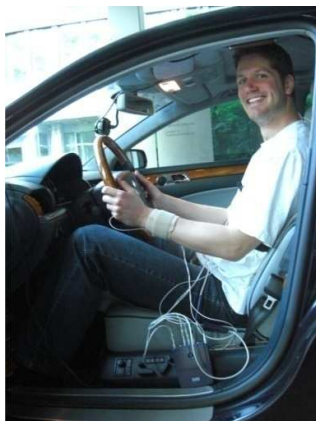
Fig. 2.: Sensor placement and connection to the NeXus-10 device attached to the side of the seat.
