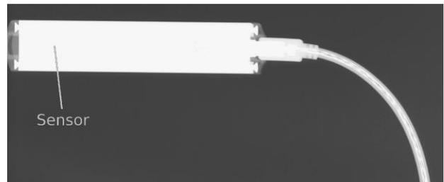
Fig. 2: Exposure of the dosimeter Xi taken with the Siemens MAMMOMAT Inspiration.
