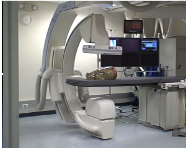
Figure 1. C-arm CBCT system used for imaging in this study.
