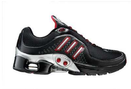
Fig. 2. The adidas 1 intelligent running shoe. It consists of a magnetic sensor element that can measure heel compression, a embedded microcontroller that performs classification and a motor which can adjust the stiffness of the sole.
