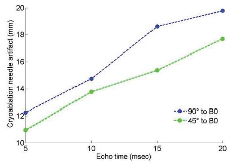
**Figure 4.** Cryoablation needle artifact (mean diameter in mm) for different TEs at 45° and 90° with respect to B0.
