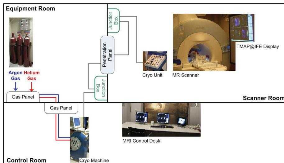
**Figure 1.** System setup visualizing the flow of argon gas for freezing and helium gas for active thawing. The flow of gas is handled at the cryo machine in the control room and the cryoablation needles are connected to the cryo unit inside the scanner room. The display of the developed thermal therapy monitoring and guidance system, called TMAP@IFE, is projected onto a screen next to the MR scanner.
