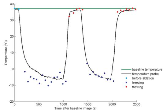
**Figure 6.** Temperature over time at a voxel close to iceball border. Both the PRF method and the temperature probe show that the temperature drops very fast but also rises rapidly during active thawing.
