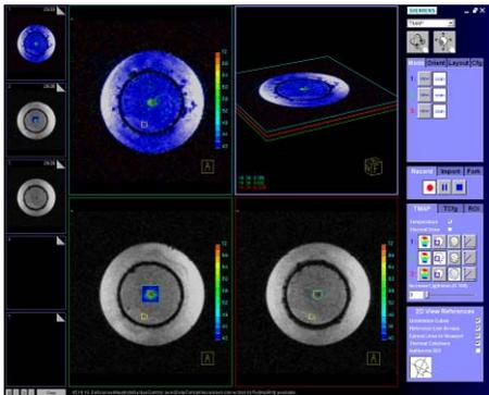
Figure 1: Cross-sectional images of a meat sample (inner circle) heated with HIFU. Basic functionality is shown including temperature overlay, region of interest selection and isotherms.
