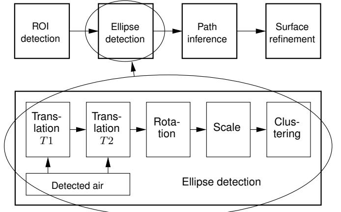
Fig. 2. Overview of the system and the steps involved in ellipse detection.
