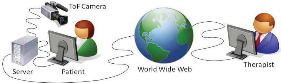
Figure 5. Schematic overview of the telemedical system (Stürmer et al. 2008)
