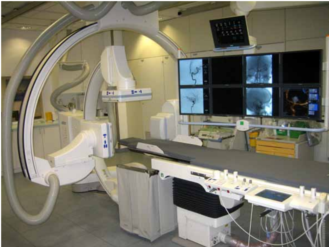
Figure 1.3: Modern C-arm system at the Department of Neuroradiology (University Hospital Erlangen, Germany) Siemens AXIOM Artis, Forchheim, Germany.
