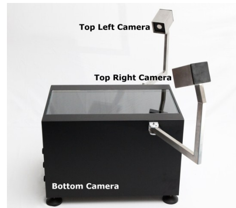
Figure 1: Proposed setup with multiple ToF cameras. The bottom camera is placed below the glass plate.
