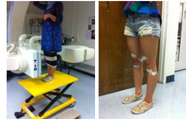
A volunteer was scanned while standing in a C-Arm CT. The C-Arm rotates in a horizontal plane. One-mm Tantalum markers were suitably attached around knee.
