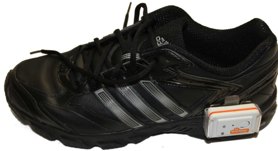
Fig.1: SHIMMER™ sensor node mounted on shoe (ankle position).
