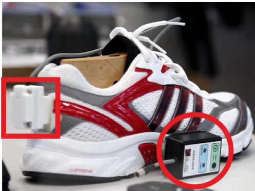
Figure 1. Inertial sensors mounted on the heel of an adidas Duramo 2 (box) and data logger (circle).
