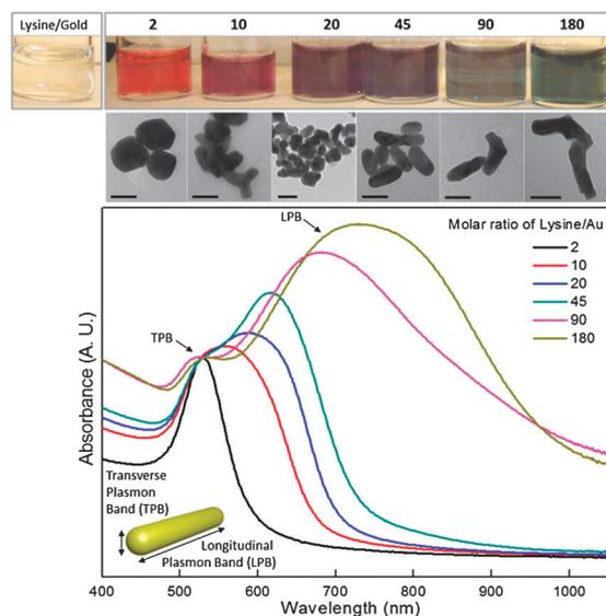
**Fig. 1** Absorption spectra and TEM images of the gold nanorods (GNRs) grown with varying amounts of the lysine/gold precursor (Lys/Au) ratio. Various colors of the GNR solutions correspond to the absorption spectra of different Lys/Au ratios (top). Corresponding TEM images showing structural evolution (middle, also see Fig. S1). Scale bar is 30 nm.
