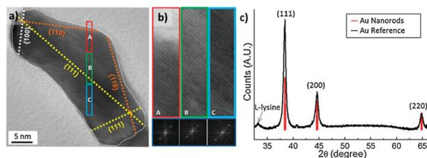
**Fig. 3** HR-TEM and XRD analysis of the gold nanorods. (a), (b) HRTEM image with lattice orientations; {111}, {100} and {110}. (b) HRTEM images correspond to the colored boxes A, B and C in (a) presented in the left. Right images show Fourier transforms of A, B and C, respectively. (c) XRD spectrum from dried bulk GNRs (black). Spectrum from reference bulk gold (red). Small sub-peak at  $33^\circ$  is attributed to crystalline L-lysine from the residue.
