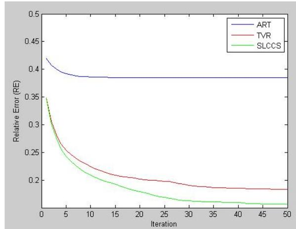
**Fig. 4.** Converge map. SLCCS converges faster than the other two method and gives best reconstruction quality
