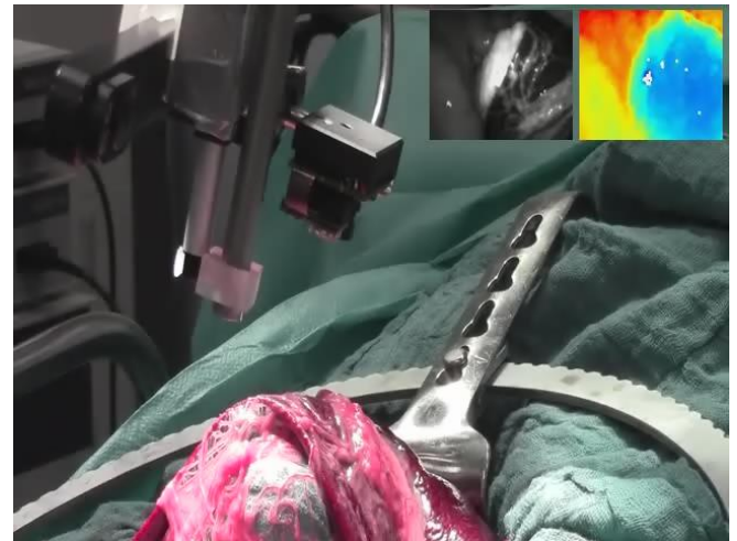
Fig. 4. The setup in an in-vivo pork study. The upper left image is a grayscale image acquired by the Time-of-Flight sensor. The upper right image is the corresponding color coded range image.
