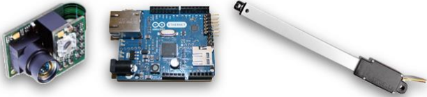
Fig. 1. The three components of our enhancement module. From left to right: PMD CamBoard nano, Arduino Uno micro controller, L12 linear servo motor.
