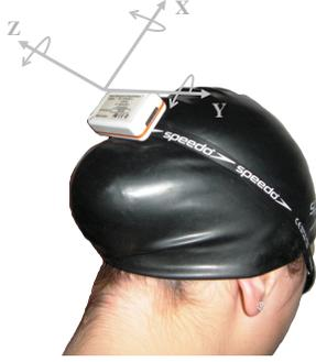
Fig. 1. Schematic sensor placement at subjects' occiput with accelerometer and gyroscope axes x, y and z.
