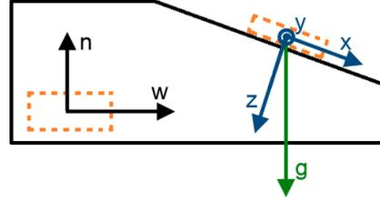
Figure 1: View on the sagittal plane of the foot symbolized by the black frame. Sensors are displayed as orange boxes with dashed lines.  $\mathbf{n}$ : normal vector of the horizontal plane,  $\mathbf{w}$ : walking direction,  $x, y, z$ : axes of sensor on instep,  $\mathbf{g}$ : gravitation vector
