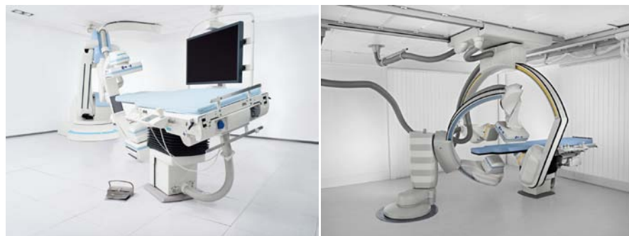
Figure 1: Typical angiography systems. The image on the left shows a C-arm system mounted on a robotic arm that is typically used in a surgical environment. The image on the right shows a biplane system as it is typically used in a neuro-surgical application.
