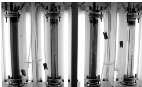
Fig.1 Photobioreactor screening modules for a batch cultivation of Porphyridium purpureum
