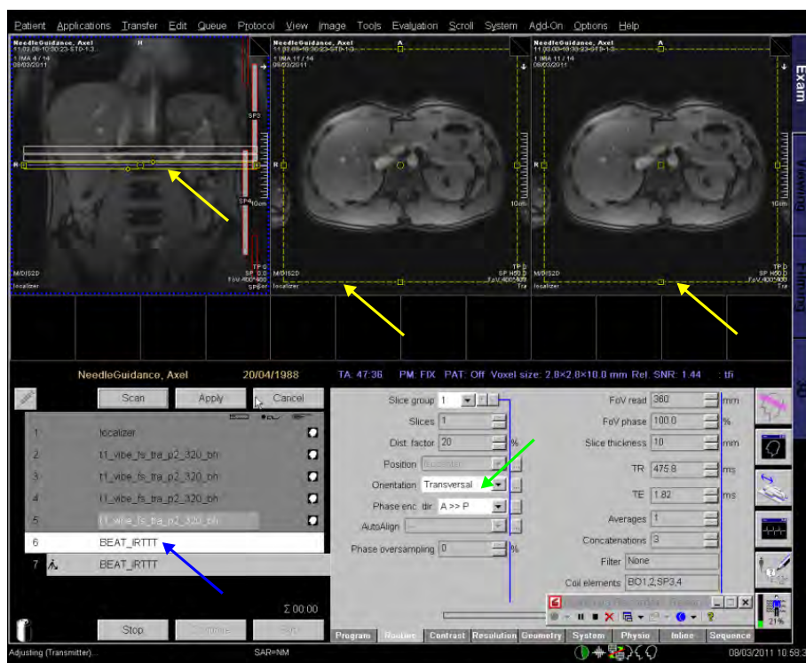
Figure 4.17: Siemens MR scanner UI with an interactive pulse sequence running (blue arrow). The displayed images are not updated in real-time which makes real-time slice alignment on the standard MR scanner UI challenging. Protocol parameters which can be changed during image acquisition are marked in white (green arrow). The user can reposition the real-time imaging slices by moving the yellow boxes in the top three viewports (yellow arrow). The developed prototype allows automatic alignment of those slices along the planned path.
