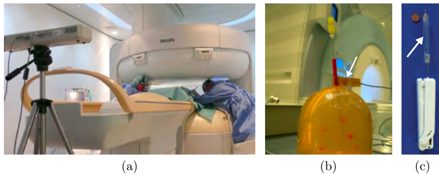
Figure 3.4: Guidance systems for needle placement inside the MR scanner bore under continuous imaging. (a) Experimental setup for optical needle tracking inside the bore for real-time image-guided needle placement. Image reproduced from [Gttl 10] with permission from Felix V. Güttler. (b) Active tracking system based on MRI gradient fields (EndoScout, Robin Medical). A sensor (arrow) with integrated miniature coils is attached to the needle. Image reproduced from [Staf 09] with permission from ISMRM. (c) Passive marker (arrow) attached to the needle is automatically tracked by a special pulse sequence. Image reproduced from [De O 08] with permission from John Wiley and Sons.
