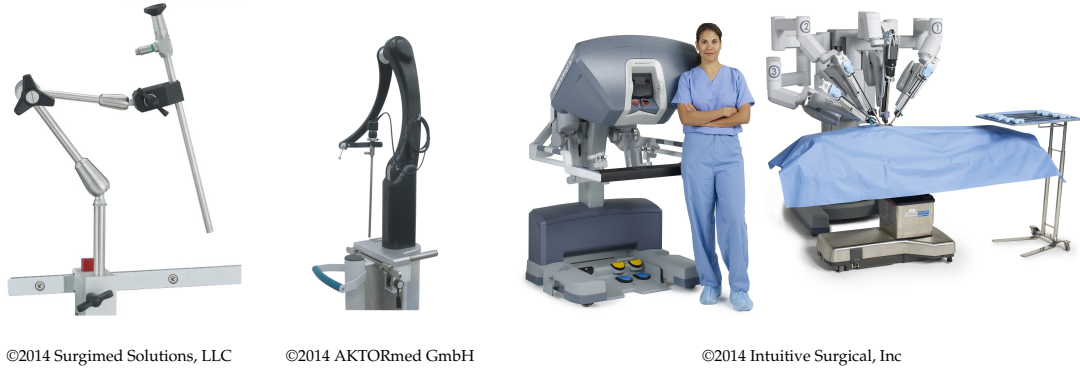
Figure 2.3: Photos of three surgical assistance systems. First, a static endoscope holder from Novid Surgical. Second, the SOLOASSIST, a joystick navigated endoscope holder. The third photo shows the da Vinci assistance system with the workstation on the left and the distant robotic system on the right.
