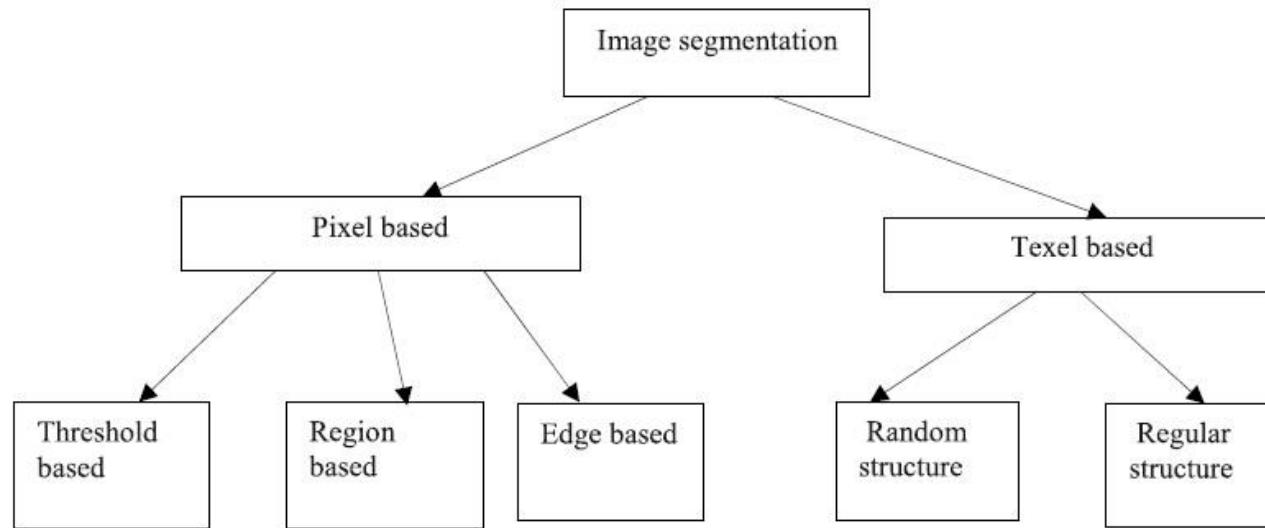
**Figure 2:** Image segmentation methods [2]
