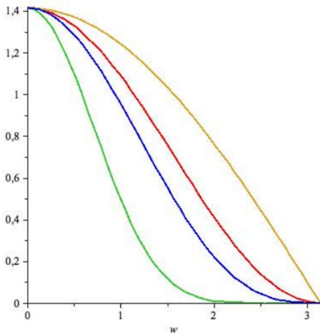
Figure: Frequency representations of the B-spline filters of length 2,3,4,8
