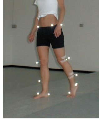
Figure 2. VICON optical tracking system with suitably placed markers to capture the motion of a lower body.
