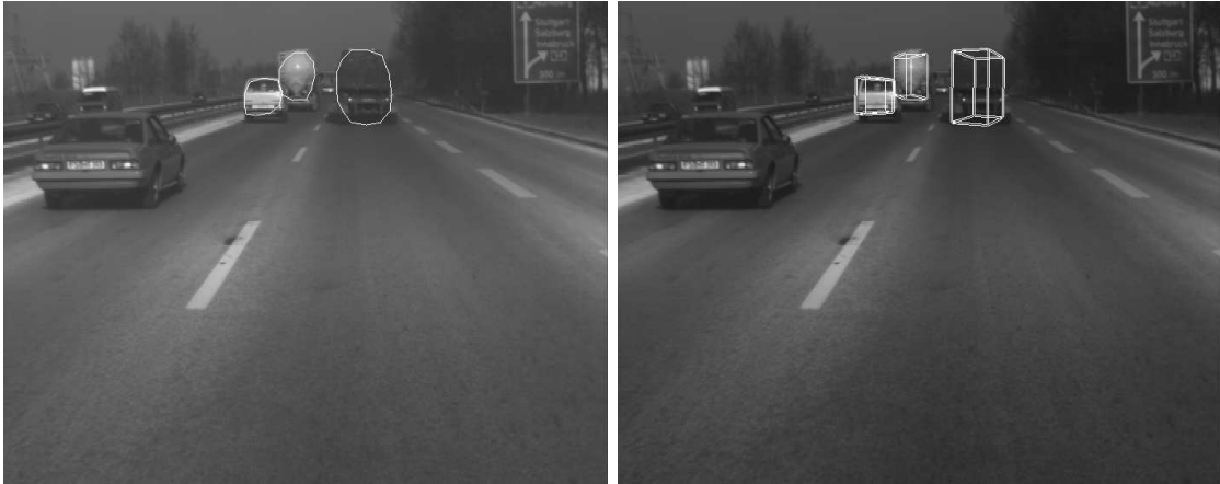
Figure 6: Results for the estimation of bounding volumes for three moving cars (right), which have been tracked by active contours (left).
