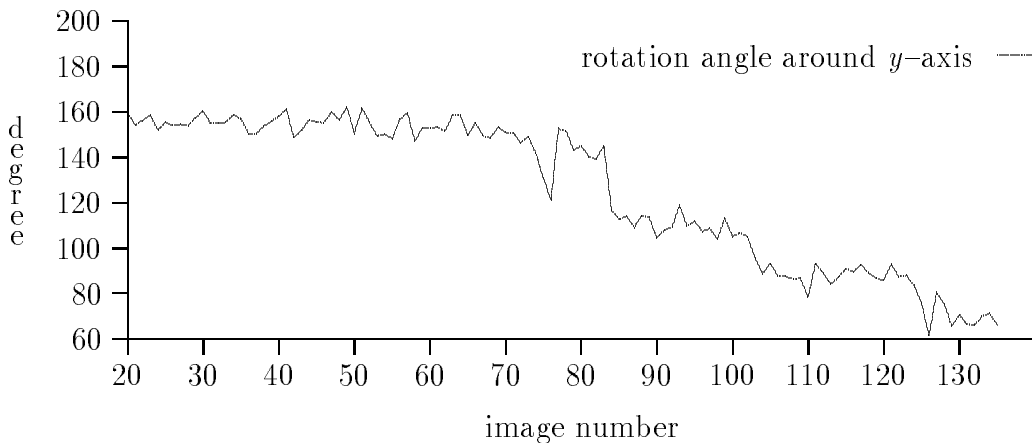
Figure 4: Calculated angle around the y -axis of the 3D bounding volume (by equation (8)) for the image sequence shown in Figure 3.
