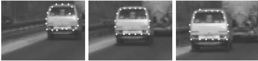
Figure 10: Results for tracking a car on a highway with active rays (images 4, 44, 84 of a sequence of 123 images taken at video rate): the sampling step size \Delta\phi is \pi/9 .
