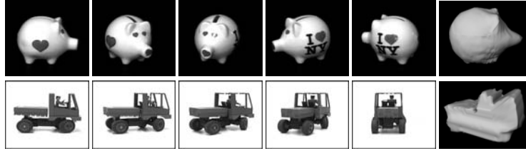
Figure9. Some images out of the sequence taken from [15] and one recorded by us, and reconstructed coarse models.
