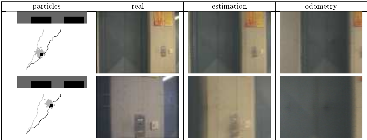
Figure 7. An experiment similar to the one shown in Figure 6 except that the used information about the robot's movement is a perturbation of the odometry. This path is drawn as a gray line. The initialization step was the same as in Figure 6, the two rows here show the situation at the 10th and the 20th frame of the test sequence.
