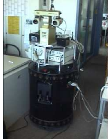
Figure 5. The autonomous moving platform with a mounted stereo head. We only use one of the cameras.
