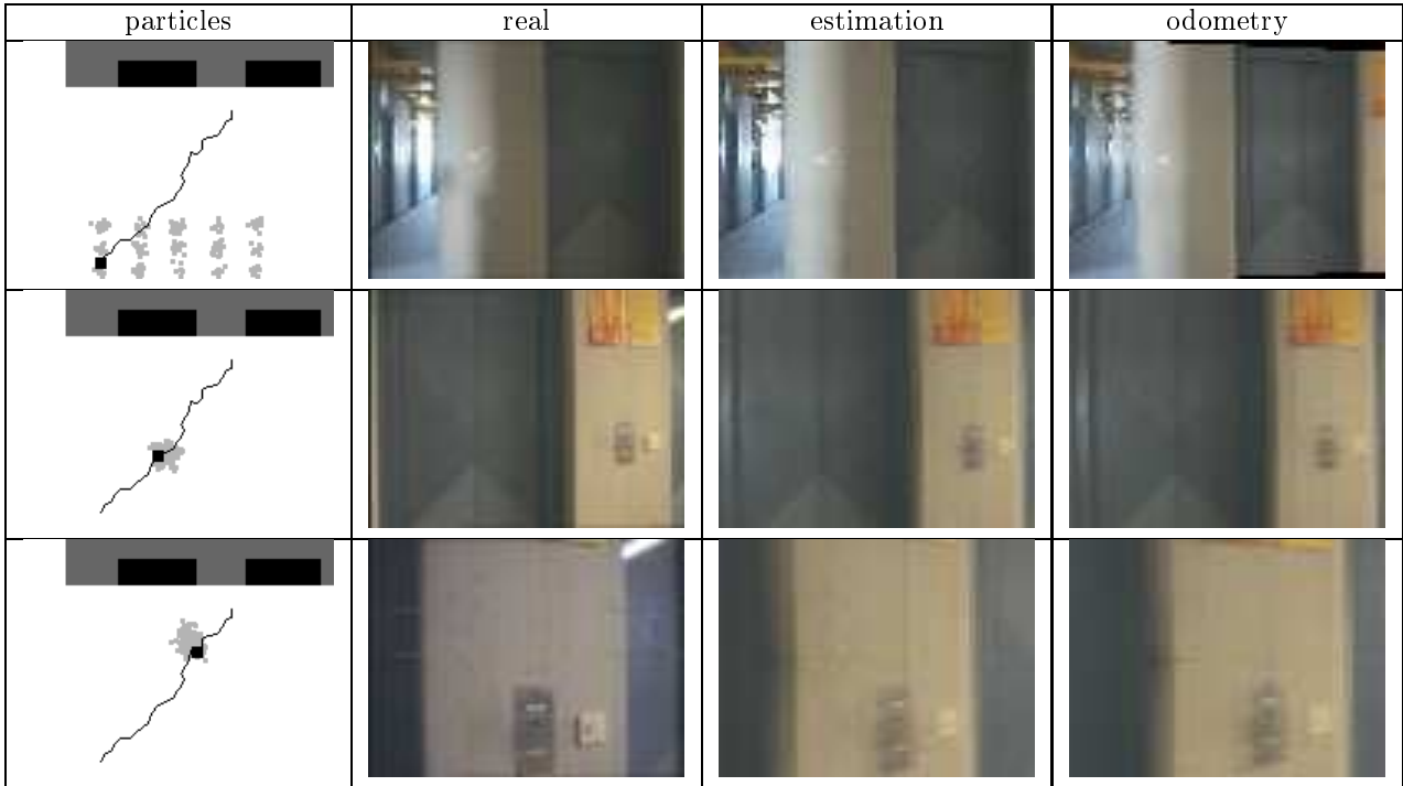
Figure 6. An experiment for testing the localization capability of our approach when using the robot's odometry. The left images show a schematic top view of the area in front of the wall (gray area) with the elevator doors (black rectangles). The positions of the particles are drawn as gray dots, the moving path as given by odometry is drawn as dark line, the actual position of the robot is drawn as a small black square. The right three images show the comparison of real camera views (left) with rendered images at the estimated most likely position (middle) and at the position which is given by odometry (right). From top to bottom, the situation at the 1st, 10th, and 20th frame of the test sequence is shown.
