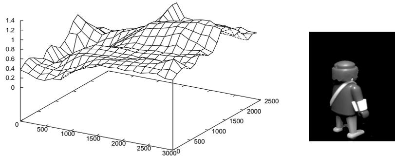
**Figure 4.** Left: MI in the viewpoint selection example assuming a uniform prior (computed by Monte Carlo evaluation). The  $x$  and  $y$  are the motorsteps for the turntable and robot arm, respectively. Along the  $z$  axis the MI is plotted. Right: best view  $\mathbf{a}$  decided by the maximum in the MI ( $\mathbf{a} = (2550, 1500)$ ). As example, object band is shown.
